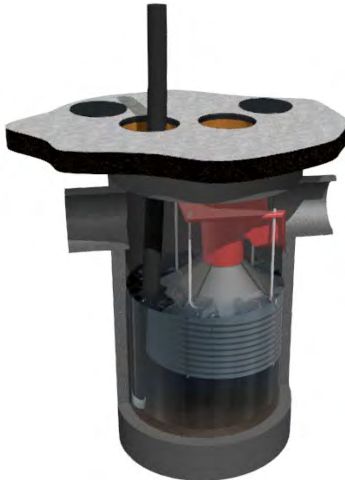
Fig.4 Floatables are removed with a vactor hose
